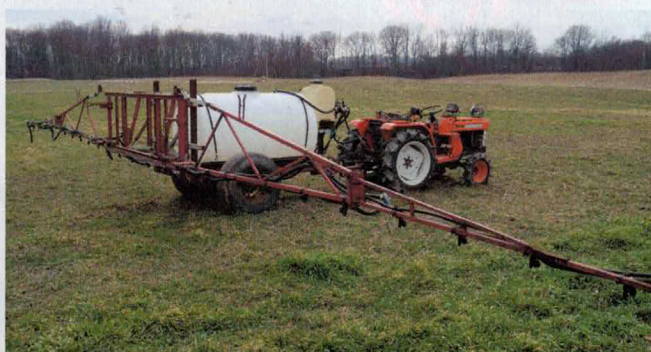
FLEXIBLE LINEUP. Greensburg, Ind., no-tiller and strip-tiller Roger Wenning uses a SpraCoupe 230 with a 60-foot boom for most of his spraying, but also utilizes a smaller sprayer with a 45-foot boom, pulled by a 19-horsepower tractor, for early burndown if a field is very wet. "This is very critical for burning down annual ryegrass," he says.
