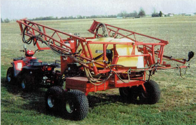
LIGHT FOOTPRINT: ATV sprayers, like this JM Innovations Mini Floater, give no-tillers the ability to get on wet ground sooner in the spring.
